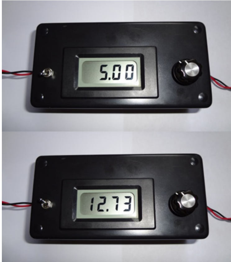
FIGURE 10 – Voltmeter showing the output (top) and input (bottom) voltage; see the positions of the switch on the left
