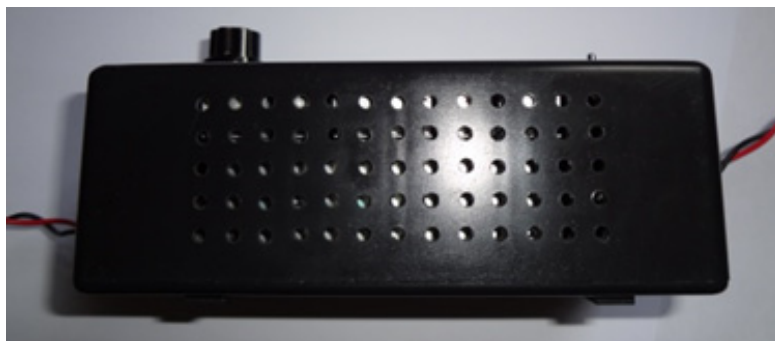
FIGURE 8 – Holes on the back of the enclosure (next to the heatsink) for proper heat dissipation
