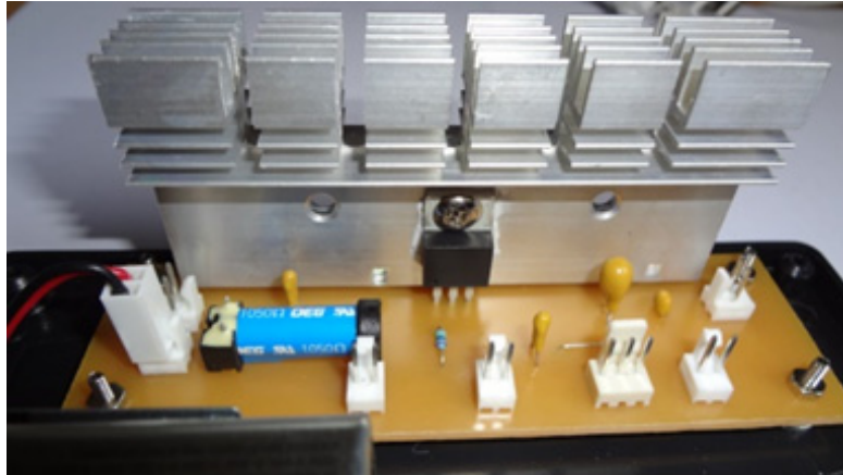
FIGURE 7 – Heatsink attached to the regulator; the reed-relay can be seen on the left (light blue body)
